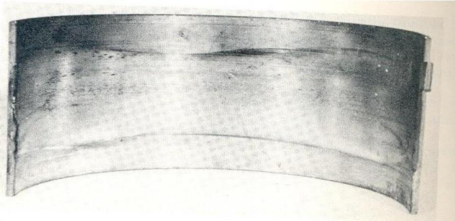
**Fig. 1-14** Bearing worn in the center by a barrel-shaped shaft.
