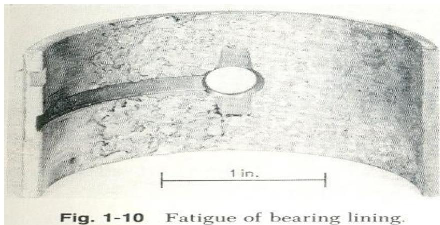
**Fig. 1-10** Fatigue of bearing lining.
