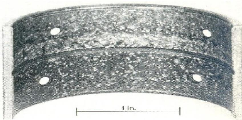
**Fig. 1-8** Bearing with severe dirt embedment.
