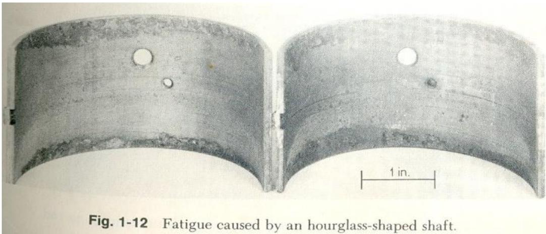
**Fig. 1-12** Fatigue caused by an hourglass-shaped shaft.
