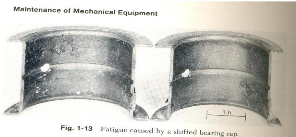
**Fig. 1-13** Fatigue caused by a shifted bearing cap.
