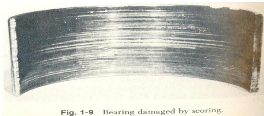
**Fig. 1-9** Bearing damaged by scoring.
