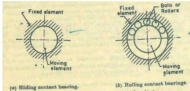
**Figure. 2 Sliding and Rolling contact bearings.**
