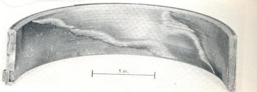
**Fig. 1-15** Skewed-wear pattern caused by a bent connecting rod.
