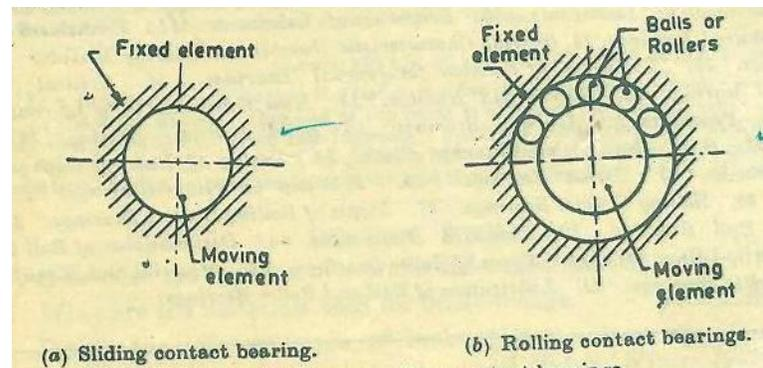
**Figure. 2 Sliding and Rolling contact bearings.**
