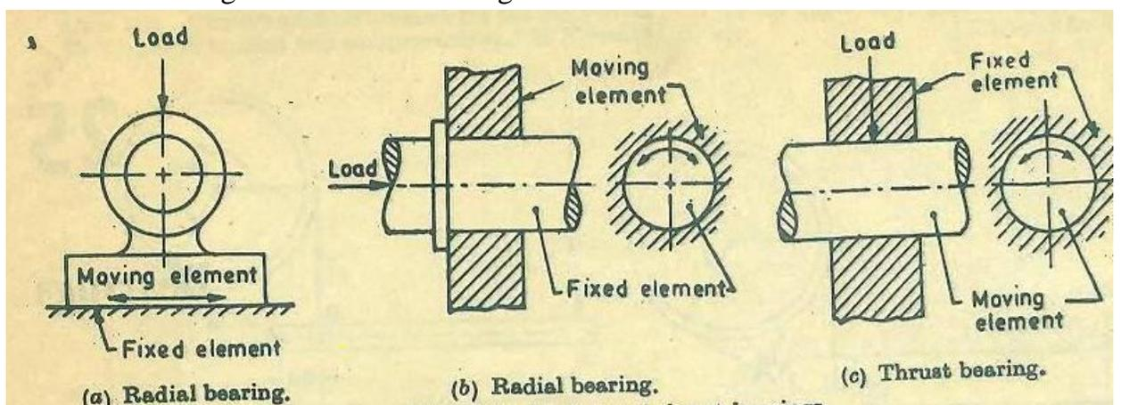
Figure 1 Radial and thrust bearings.
