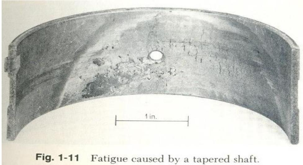
**Fig. 1-11** Fatigue caused by a tapered shaft.
