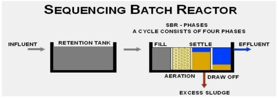
Various Phases In a Typical SBR Process
