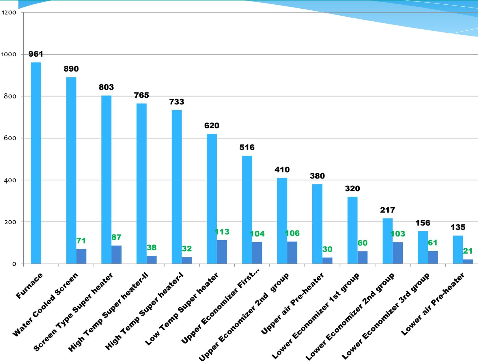
**Thermodynamic aspect of Flue – gases in HP Boiler for control measures Temp (oC)**
